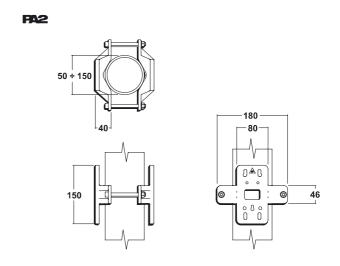
PA1 and PA2 are compatible with camera housing Linea 1,Linea 2,Linea 6, Linea R and illuminators Hyperion and Hyperion One.
